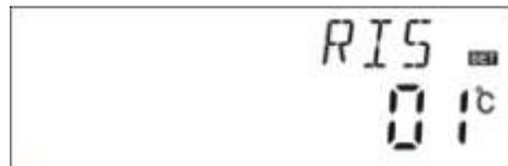
▶ Press “+”“-” button, to adjust increase rate of (RIS) of temperature difference, adjustable range (1°C~20°C), factory set is 1°C
