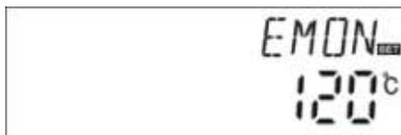
☀️ ⓘ These two signals display on the screen, means collector emergency switch-off function is activated, and tank temperature rises up to its maximum permitted temperature.
