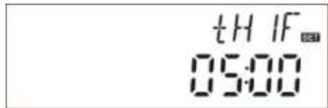
▶ Repress “SET” button, “00” of minute time blinks on screen
