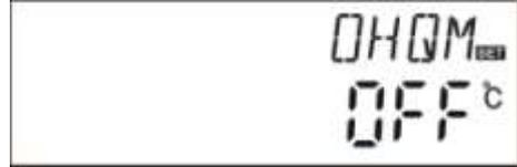
▶ Repress “+”“-” button, to activate this function, “OHQM oN” blinks on the screen
