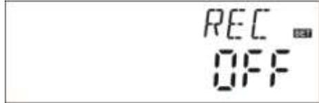
▶ Re-press “SET” button to activate or deactivate this function, after function activated; factory set is “REC ON”
