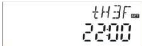
**Note:** when no gas or oil boiler is installed in system, electrical heater can be installed as back-up device, when electrical heater is in operation status, signal
