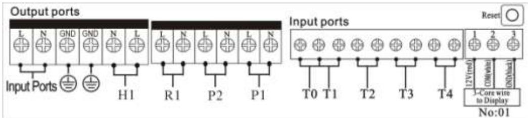
“**Reset**” button: This button is on the terminal connection panel, when system program is out of working, press “Reset” to recover the program of system to the factory settings.
